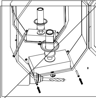
5. Secure the bottom of the product to the wall using wall by lining up the product's location holes to that of the mounting screws. Ensure the product is safely secured. Remove the product from the wall, pre-drill the holes and install the wall plugs.
