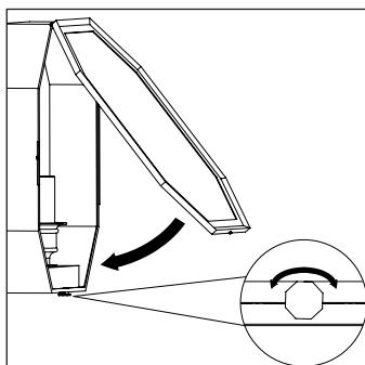
7. After accessing the bulb, gently close the door. Close the latch and ensure it is secure.
