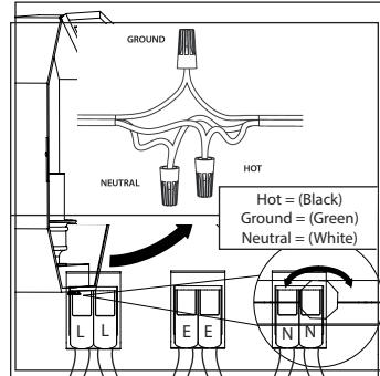
6. To access the bulb, twist the hatch to release the door hold wiring, connect the building supply and the product cables together in the wire connectors as shown above.
