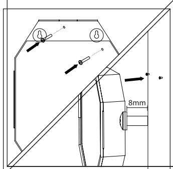
4. Position the product onto the wall by lining up the product's fixings prior to installation. Position screw holes in a suitable location around the box. Screw suitable fixings to the two top mounting locations.
