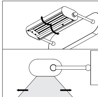
4. Locate the household wiring and feed through the centre of the back plate.
