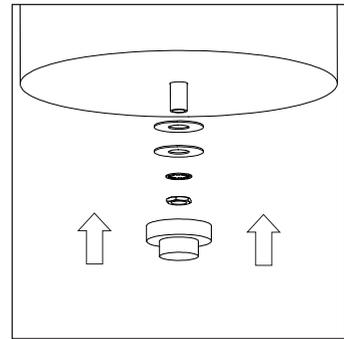
6. Replace the decorative bowl and re assemble the rubber washer, washer, nut and finial in this order. Ensuring all component are tightly secured. Caution should be taken to support the decorative bowl at all times.
