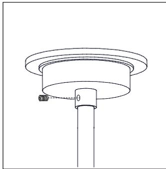
5. Secure the ceiling rose cup to the ceiling using the grub screw, ensuring it is tightly fitted
