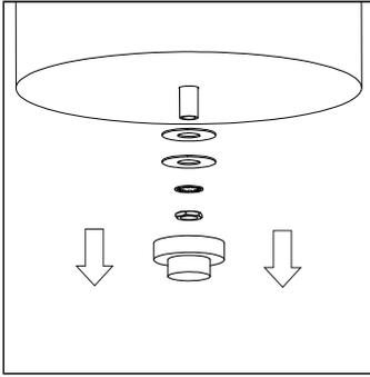
1. Holding the decorative bowl, unscrew the finial, and remove the nut, washer and rubber washer.
