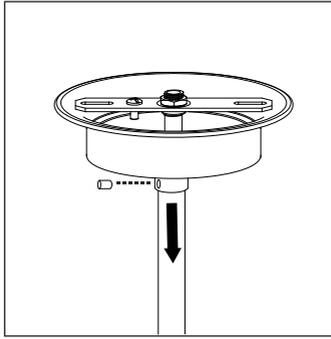
2. Loosen the grub screw to drop the ceiling rose.
