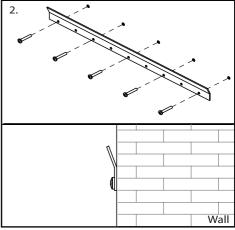
Use the screws provided to mount the Z Bar so that the top of the Z Bar is away from the wall. Ensure the Z Bar is secure.
