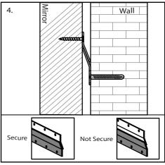
Make sure the mirror is stable and securely fitted before releasing the mirror.
