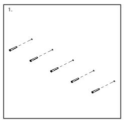
At the desired install location, mark and drill holes using the Z Bar as a guide. Ensure the Z bar is level. Insert the wall plugs into the mounting surface.
