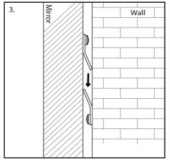
Carefully slide the mirror over the top of the Z Bar mounted to the wall, so the two Z Bars align & connect.
