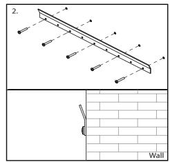
Use the screws provided to mount the Z Bar so that the top of the Z Bar is away from the wall. Ensure the Z Bar is secure.
