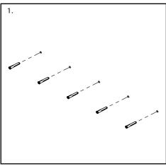
At the desired install location, mark and drill holes using the Z Bar as a guide. Ensure the Z bar is level. Insert the wall plugs into the mounting surface.
