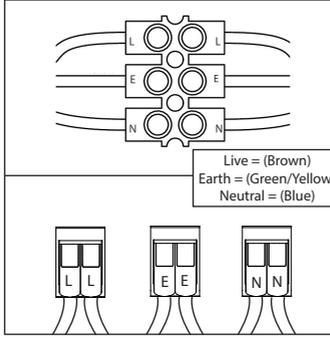
2. Having identified the household wiring, connect the building supply and the product cables as shown above.
