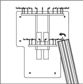
4. Starting with the lower tier, attach the glass onto the frame.
