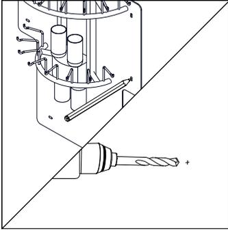
1. Mark and drill location holes in the mounting wall, based on mount holes on the product.
