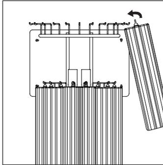
5. Attach the remaining glass onto the upper tier.
