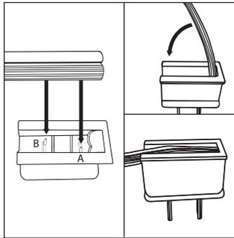
8. Using the extra plug provided. Line up the cable so that the ribbed side lines up with pin A and the smooth side to pin B. Push the cable down into the cable hole as far as possible and bend the cable onto the metal pins, piercing the cable.
