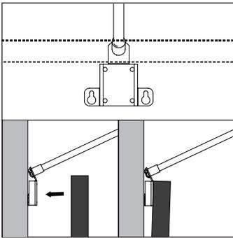
1. Decide where to mount the product. For wall mounting, line the product up with the picture frame as shown. Take consideration for how much the picture drops when hung up.
