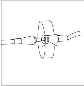
5. Connect the light and the LED driver using the D.C supply connector.
