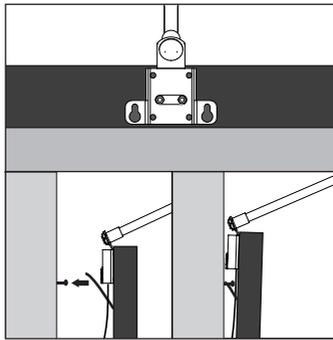
2. If mounting onto the picture, Line the product up to the frame as shown. Ensure the screws line up with the frame to avoid any damage from the screws.
