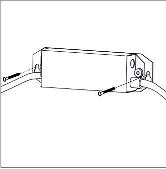
4. Attach the LED Driver to the wall using suitable fixings. Please note the led driver is external from the light fitting and must be accommodated during installation.
