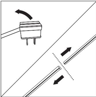
7. To change the plug cable length, unplug the product and remove the plug supplied and cut the cable to the desired length.
