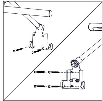
3. Mount the product using the screws provided to the wall or picture frame.
