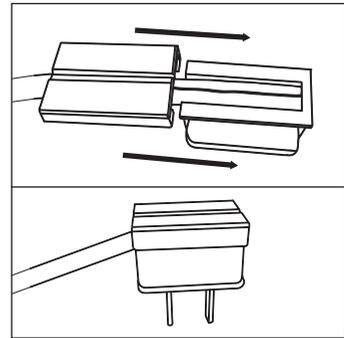
9. Slide the cap onto the top of the plug securing the cable.
