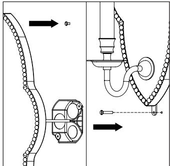
4. Hang the product on the wall using the mounting bracket. Ensure it is hanging straight. Secure the product to the wall using the fixng hole/s.
