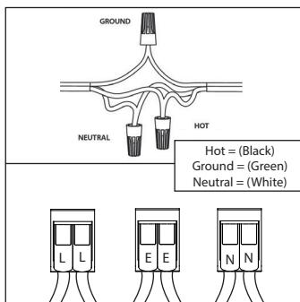
4. Having identified the household wiring, connect the building supply and the product cables together in the wire connectors as shown above. Ground connection can be found on the ceiling bracket.
