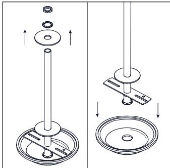
1. The product must be installed to a structural support suitable for the weight of the product. Ensure you have access to the top of the mounting support. Drill a hole through the support and remove the nuts, the lock washer, the large washer, and ceiling rose. Ensure the remaining washers and nut are far enough down the tube to allow the tube to be fitted the whole way through the mounting support.
