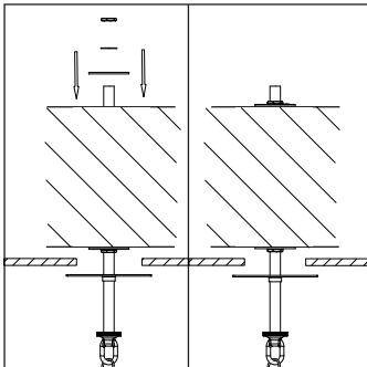
2. Push the bar through the structural support, keeping the bracket below the ceiling. Reattach the components removed in the previous step above the support and ensure they are secured tightly.
