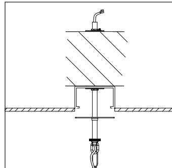
3. Thread the cable through the ceiling loop and into the threaded tube until it comes out above the support.
