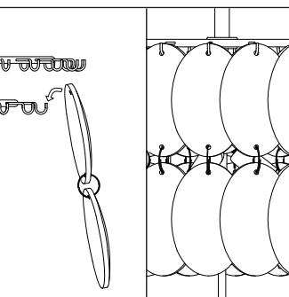
8. Lift the glass up and hang on the hook using the hole located at the top of the glass. Continue hanging the glass petals so they overlap the previous one. Begin by hanging the petals from the central hooks first, before moving on to the outer hooks. Complete loading of glass onto 1 tier before starting the next tier, so to avoid product becoming unbalanced.
