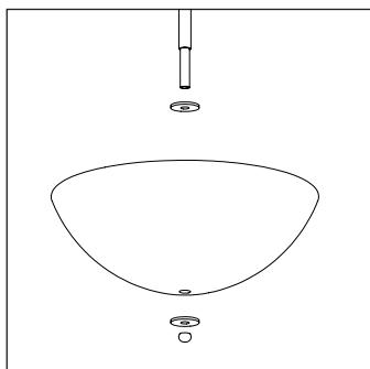
7. Carefully attach the glass bowl to the base of the light using the finial and washers provided.
