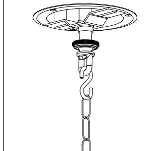
3. Attach the chain to the ceiling bracket loop.
