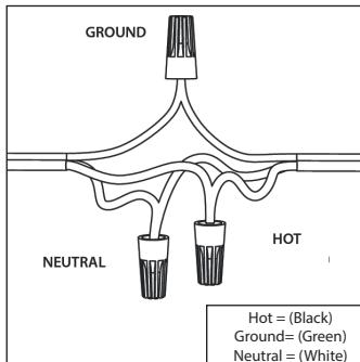
4. Having identified the household wiring, connect the building supply and the product cables together in the wire connectors as shown above. 3/8 of bare conductor should be exposed for the terminations.
