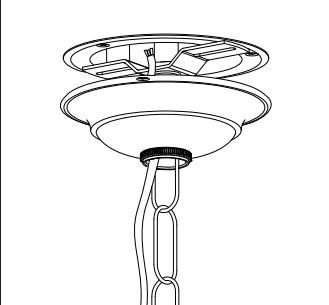
2. Thread the cable through the chain, ceiling rose cup and loop.
