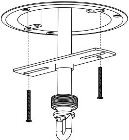
4. Attach the bracket to the Ceiling Box ensuring it is secured tightly.
