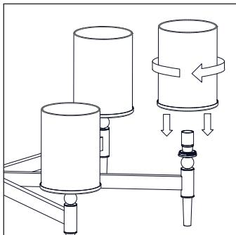
7. Screw the glass diffusers onto each arm, ensuring they are secured tightly. Repeat this step from each side to keep the weight evenly distributed.
