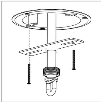
5. Attach the bracket to the Ceiling Box ensuring it is secured tightly.
